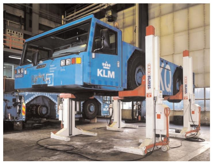
The flagship of our program is the mobile column lift, which is available with lifting capacity from 10,000 lbs. / 5.500 kg. up to 40,000 lbs. / 17.500 kg. per column. The advanced Stertil-Koni mobile column lift has earned its popularity because it has cleared the way for efficient and flexible workshop management.
