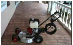
Have clients or prospects with wooden decks? The Mystic Washer® offers a variable psi control so you can 'dial it in' for the amount of pressure needed for wooden or other decking. There is no better, easier or more cost-effective way to clean decking than with the Mystic Washer®.
