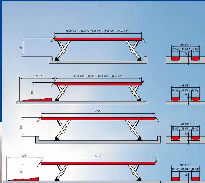
\* Flexible measurements dependent on customer requirements
