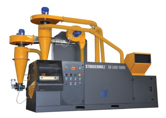
The Stokkermill 5000Turbo is with added TURBO function, ideal for medium to large recycling companies which processe large quantity of cables. Expansion as adding pre-grinders and automatic conveyor delivery systems with or without magnet seperation.
