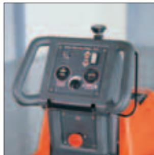
All control elements including ground pressure adjustment in direct access. The variable handlebar guarantees fatigue-free working.
