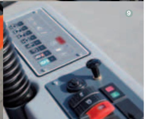
The Jonas 1500 cockpit can be accessed easily from both sides. Clear view of the side brushes at the front. The particularly simple operating concept ensures the user does not get confused. The entire sweeping function can be switched on and off with just one button ⑨. Customers can define individual programmes.
