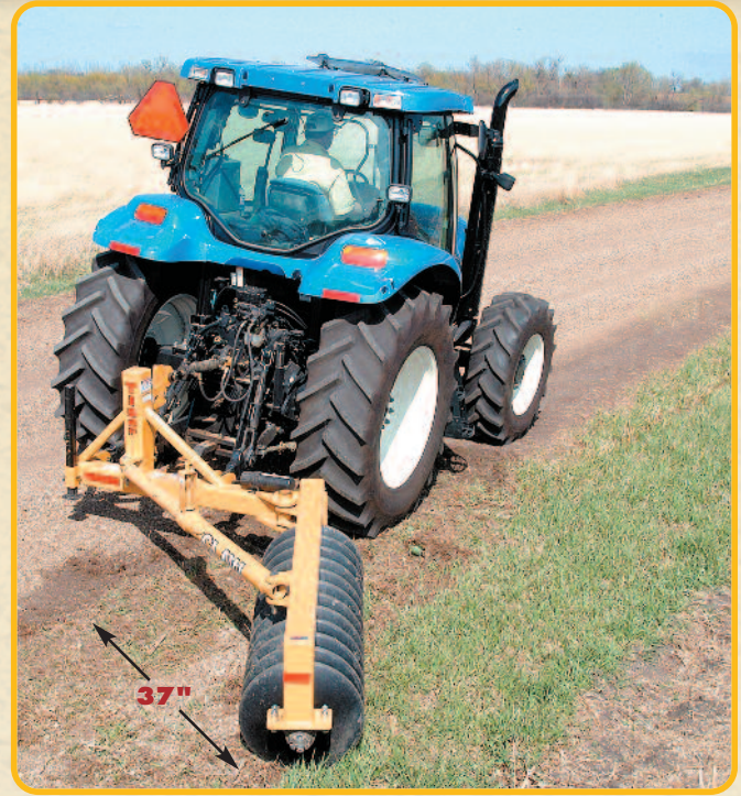
Patented angle design effectively moves and mulches 37" of material.
