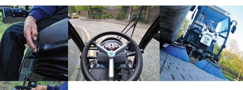
**Suspension:** From the ground up, the design of the CN101 is focussed on 'driver ride'. The chassis features independent coil springs and dampers to the front and rubber cone suspension at the rear combined to give a smooth ride, low vibration and stable curb climbing.
