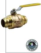
The APOLLOXPRESS™ 77W Series Press End Ball valve is designed for direct mechanical connection to ASTM B88-Type K, L, and M copper tubing in the hard drawn condition. The 77W is ideal for installation in most plumbing and heating systems, including potable water. Now with Leak Before Press™ feature and 250 psig maximum working pressure. Lead free option available.
