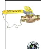
The APOLLOXPRESS™ 77W-HC Press x Hose ball valve is designed for direct mechanical connection to ASTM B88-Type K, L, and M copper tubing in the hard drawn condition for sizes 1/2"- 3/4". Valves feature a 3/4" hose connection with heavy brass cap to protect the threads. The 77W-HC is ideal for most plumbing and heating systems, including potable water. Now with Leak Before Press™ feature and 250 psig maximum working pressure. Lead free option available.
