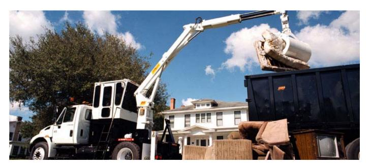
Great system for high volume route collection. The most advanced and efficient system for collecting trash on the market. Two features that set this unit apart are the ability to drive in reverse from the operator's station and not needing outriggers for most loading operations.
