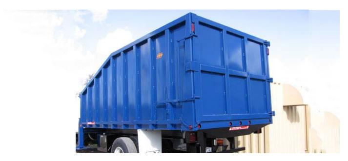
Petersen's model TBH trash dump body was designed for heavier operations like sidewalk removal, large stumps and C&D waste. Heavy duty style body is also mandatory for higher volume bodies.
