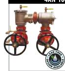
Double Check Valves in an "n" flow pattern in sizes 2-1/2"-12". Stainless steel bodies 2-1/2"-8", FDA-Approved epoxy-coated ductile iron 10" and 12". Patented TriForce™ checks in all sizes for low head loss and small footprint. Available shutoffs: monitored butterfly valves with supervisory switch, OS&Y and NRS gate valves. Vertical up/vertical down installation approvals.
