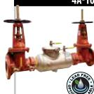
Double Check Valves in sizes 2-1/2"-12". Stainless steel bodies 2-1/2"-8", FDA Approved epoxy-coated ductile iron 10" and 12". Patented TriForce ™ checks in all sizes for low head loss and short lay length. Available shutoffs: monitored butterfly valves with supervisory switch, OS&Y and NRS gate valves. Horizontal and vertical installation approvals.
