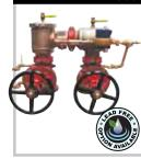
Double Check Detector Assemblies in "n" flow pattern in sizes 2-1/2"-12". Stainless steel bodies 2-1/2"-8", FDA-Approved epoxy-coated ductile iron 10" and 12". Patented TriForce™ checks in all sizes for low head loss and small footprint. Available shutoffs: monitored butterfly valves with supervisory switch, OS&Y and NRS gate valves. Vertical up/vertical down installation approvals.
