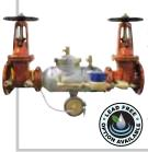
Reduced Pressure Detector Assemblies in sizes 2-1/2"-12". Stainless steel bodies 2-1/2"-8", FDA Approved epoxy-coated ductile iron 10" and 12". Patented TriForce ™ checks in all sizes for low head loss and short lay length. Available shutoffs: monitored butterfly valves with supervisory switch, OS&Y and NRS gate valves. Horizontal installation approvals.
