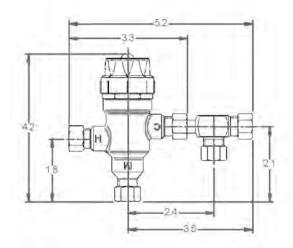
The Apollo<sup>®</sup> MVD (34D Series) Mini Thermostatic mixing valves are designed for ASSE 1070 "Point of Use" temperature control applications with a single fixture using proven ASTM grade materials. These valves will hold a desired temperature within  $\pm$  3°F and will shut off flow in the event of hot or cold water failure. They come equipped with a tamper-resistant high temperature limit stop to prevent adjustment above 120°F.
