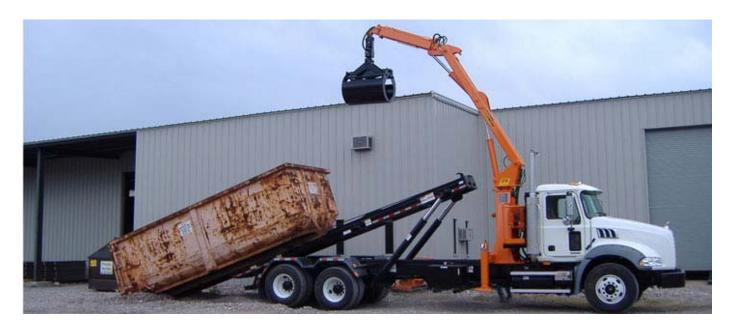
The model BL-3 is a 20 ft. knuckleboom loader that is permanently mounted in front of a roll-off. You can use your existing roll-off boxes with this system.
