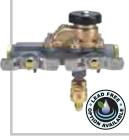
Spill-resistant pressure vacuum breaker (SVB) is designed to prevent contamination of potable water due to back-siphonage and is ideally suited for indoor and OEM applications supplied with continuous pressure where water discharge could cause problems. Full USC-FCCC&HR, ASSE, and CSA approvals. Sizes 1/4" to 1/2" Noryl® body.
