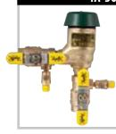
Bronze body pressure vacuum breaker with internal freeze relief valve and captured spring cartridge. Features Apollo® ball valve shutoffs with stainless steel handles and trim. Full USC-FCCC & HR, ASSE, and CSA approvals. Sizes 1/2"-2".
