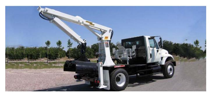
The rear-mounted RL-3 is designed for loading into attached trailers or into separate haul trucks.
