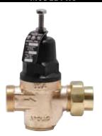
Handles supply pressures up to 400 psig; working temperatures to 180°F. All-bronze body, corrosion resistant cage, stainless steel strainer and seat. Meets **ASSE** and **CSA** standards; listed with **IAPMO.**
