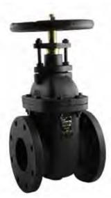
Compatible with ANSI 250# & 300# Flanges Full Port Bronze Mounted Seat Rings Solid Wedge Adjustable Graphite Stem Packing Non-Rising Stem Flanged Connection Bolted Bonnet Rugged Iron Hand Wheel Back Seat Protection **STANDARDS: MSS SP-70** "Gray Iron Gate Valves Flanged and Threaded" **ASME B16.10** "Face-to-Face and End-to-End Dimensions of Valves"
