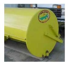
Gator Getter<sup>™</sup> was designed to be used as fast speed highway debris removal equipment. This equipment works by scooping up debris as you are driving down the road. At regular speeds, it will push the item up and around the barrel to a collection tray which will hold it until emptied. The most important virtue will be the safety significance of not having personnel in the road to remove debris in a traffic stream, no road shut downs, no traffic slow downs.
