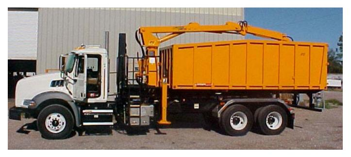
The model HL-3 is a loader and body that can be used on a hooklift truck. Adds new capabilities to your truck without having to dedicate it full-time. Minimum rail length of 19 ft.
