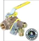
Water heater shutoff/thermal expansion control valves provide both water heater shutoff and code required thermal expansion protection. The 78-RV combination valves are offered in three pressure settings, 125, 100 and 80 psig. Available in 3/4" size with sweat, threaded and pex connections. Various relief valve connections available. CSA and IAPMO listed.
