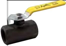
Carbon steel unibody ball valve; CWP rated 1500 to 2000 psig, cold, non-shock. Optionally meets API 607 fourth edition fire safe standards. Sizes 1/4" to 2".
