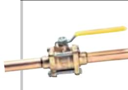
Three piece full port valve with brazed tubing. This valve is useful in pharmaceutical, medical gas and pneumatic applications where valves should not be disassembled prior to soldering or brazing.
