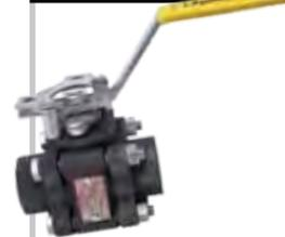
Carbon steel, full port three piece ball valve. 1500 psig CWP; stainless ball and stem, ISO 5211 mounting pad, stainless enclosed fasteners and topworks. Multi-piece V-ring packing, gland plate style packing adjustment and lockable. Available with threaded, socket weld and butt weld ends. Sizes 3/8" to 2". Limited options.
