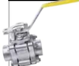
Stainless steel, full port three piece ball valve. 1500 psig CWP, ISO 5211 mounting pad, enclosed fasteners, multi-piece V-ring packing, gland plate style packing adjustment and lockable. Available with threaded, socket weld and butt weld ends. Sizes 3/8" to 2". Limited options.
