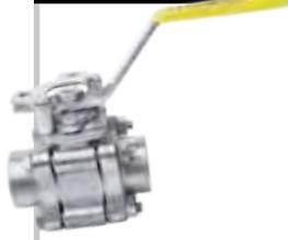
Stainless steel, full port three piece ball valve. Class 600; ASME B16.34, (all sizes), ISO 5211 mounting pad, enclosed B8M fasteners, stainless topworks, multi-piece V-ring packing. Gland plate style packing adjustment, static grounding, spiral gaskets and lockable. Available with threaded, socket weld and butt weld ends. Sizes 3/8" to 2". Numerous options including live-loading or tested to API 607 5th edition.
