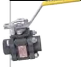
Carbon steel, full port three piece ball valve. Class 600 (all sizes); stainless ball & stem, ASME B16.34, ISO 5211 mounting pad, enclosed B8M fasteners, stainless topworks, multi-piece V-ring packing. Gland plate style packing adjustment, static grounding, spiral gaskets and lockable. Available with threaded, socket weld and butt weld ends. Sizes 3/8" to 2". Numerous options including live-loading or tested to API 607 5th edition.
