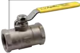
Stainless steel unibody ball valve; CWP rated 1500 to 2000 psig; optionally meets API 607 fourth edition fire safe design standards; available with "tee", round, and cam lock handles.
