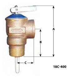
Automatic temperature and pressure relief valves feature unique non-metallic coating which protects the element against galvanic and electromechanical corrosion by isolating it from the heated water. This coating is electrostatically applied for uniform coverage, then thermobonded, resulting in optimum adhesion for extended service life.
