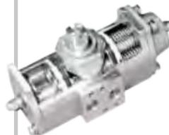
Apollo AcuTorque actuator is manufactured with an integral internal air manifold. Valve interface dimensions are ISO 5211 standard. The solenoid mounting pad and slotted shaft are manufactured to NAMUR dimensional standards. For applications not requiring a direct mount solenoid valve, ports are NPT threaded. Investment cast steel body and unique drive pinion make the AcuTorque an excellent choice for tough applications. Torque outputs from 21 to 20, 929 lb-in.
