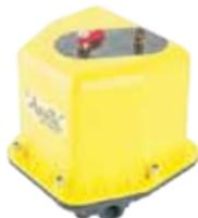
Electric actuators; torque output 200 to 1,000 lb-in, NEMA 4 & 4X (water tight and corrosion resistant) enclosures. Thru shaft manual override. Reversing motors in 24, 115, 220 VAC and 12 and 24 VDC. CSA listed.
