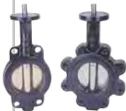
General purpose/economy ductile iron design for use in industrial and HVAC/mechanical markets. The WD141 Model is a wafer style valve; the LD141 Model is a companion lug. Both are rated at 200 psig bubble-tight shut off between flanges. LD/WD 141 Series meet MSS SP-67 and API 609 specifications. Lug sizes 2" to 24". Wafer sizes 2" to 12".
