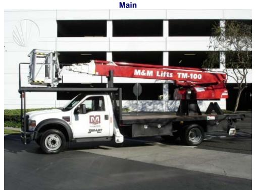
ReachMaster, Inc. proudly introduces the new TM-100 truck mounted aerial lift. The TM-100 is the first 100 foot telescopic aerial lift to be mounted on a 19,000 GVW chassis of your choice.
