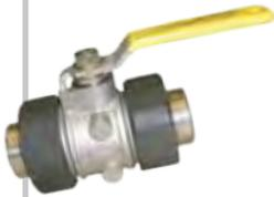
Stainless steel ball valve with double union ends; blow-out proof stem, all wetted metallic parts are 316 stainless steel. RPTFE seats and seals, adjustable packing gland and stainless steel lever and nut. Sizes 1/2" to 2".
