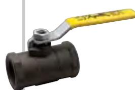
Compact bar stock steel unibody ball valve. Certified fire safe with graphite packing; RPTFE seats and seals, blowout-proof stem design. Sizes 1/4" to 2".
