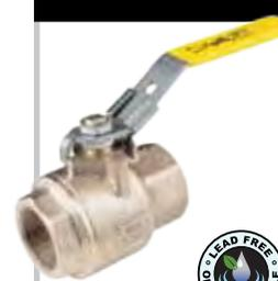
Full port "Contractor Series" bronze ball valve with solid chrome-plated ball for superior flow characteristics. U.S. made cast bronze body and retainer. NPT and ANSI B16.18 solder end connections available. Sizes 1/4" to 2-1/2".
