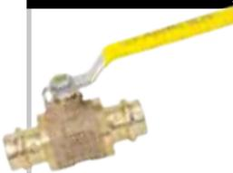
ApolloXpress™ ball valves are designed for direct mechanical connection to copper tubing in sizes 1/2"-2". The 77W complies with ANSI/NSF 61 Section 8 and is ideal for plumbing and heating systems. The press connections ensure easy installation with standard crimping tools. Rated 250 CWP, now with Leak Before Press™ feature.
