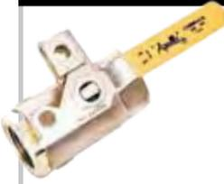
Bronze padlockable ball valve; rated 600 psig CWP; stainless steel lever and nut optional. Automatic drain available. Sizes 1/4" to 2".
