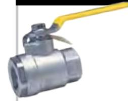
Economy stainless steel full port valve, 1000# CWP rating. Threaded ends, blowout proof stem, investment cast body, 316 SS components, including stainless handle. RPTFE seats and long life MPTFE packing. Sizes 1/4" to 2".
