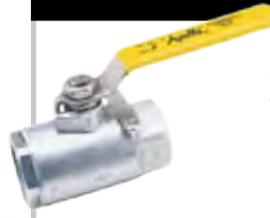
Stainless steel standard ball valve; investment cast components. 2,000 CWP to 1", 1,000 CWP 1-1/2" to 3". Sizes: 1/4" to 3". 76-600 Series - Stainless steel 3-way diversion ball valve; 800 psig WOG, investment cast components.
