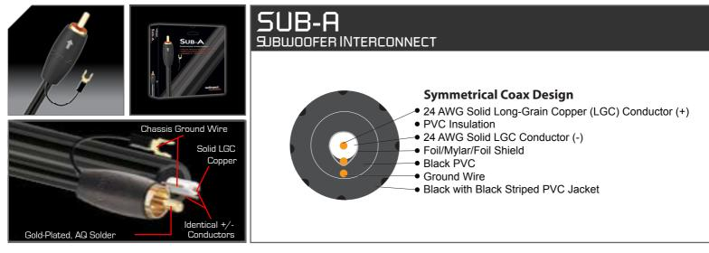
Sub-A minimizes distortion by using identical solid Long-Grain Copper conductors for "+" and "-". Solid conductors eliminate distortion caused by strand interaction. The simpler grain structure and fewer impurities within Long-Grain Copper provide significantly clearer sound than normal OFHC copper. Gold-plated high-conductivity plugs are attached with specially formulated AQ Solder.
