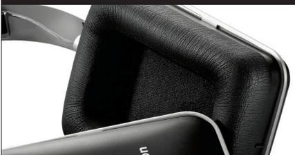
Premium foam in the ear pads contributes to the NC headphones' excellent passive-noise reduction and extended bass response. The slow-retention foam helps maintain an acoustic seal around the ear, which keeps outside noises out and also keeps the listener's music from disturbing others.
