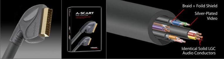
**VIDEO:** All the video conductors use solid Silver-Plated Copper (SPC). Silver-Plating greatly improves high frequency performance for a fraction of the cost of solid silver. Nitrogen Injected Hard Cell Foam insulation (HCF) reduces distortion caused by the insulating material, and helps maintain a stable 75W. The combination foil and braid shield provides 100% protection.
