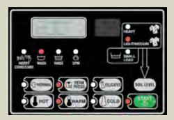
Quantum™ Control Features: Digital display for vend price and cycle time countdown. Touch pad control with LEDs. Three temperature selections for Hot, Warm or Cold water. Three fabric selections for Normal, Permanent Press or Delicate. Extra-large capacity with small load optional. Push-to-Start activation. Infrared programming.
