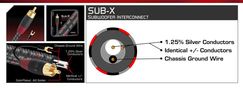
SUB-X uses two identical solid 1.25% Silver conductors for positive and negative. Solid conductors eliminate strand-interaction distortion. Foam PE insulation minimizes information smearing. A 100% coverage shield insures noise-free performance. Gold-plated high-conductivity brass plugs are attached with specially formulated AQ Silver Solder.
