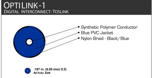
When using a Toslink (EIA-J) fiber optic cable, it is the "one" most important audio cable in your system. The sound quality of all the channels, whether two or five or more, are dependent on this one cable to deliver an undistorted, smooth, clear and dynamic performance.
