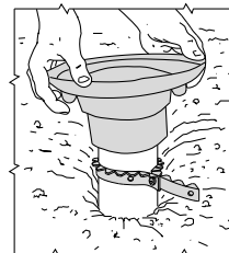
Inside Caulk Body Slips Over Stub and Rests on Support Strap
