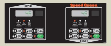
Quantum™ Control Features: Digital display for vend price and cycle time countdown. Touch pad control with LEDs. Four cycle and heat selections, dedicated Push-to-Start pad for safe operation. Infrared programming.
