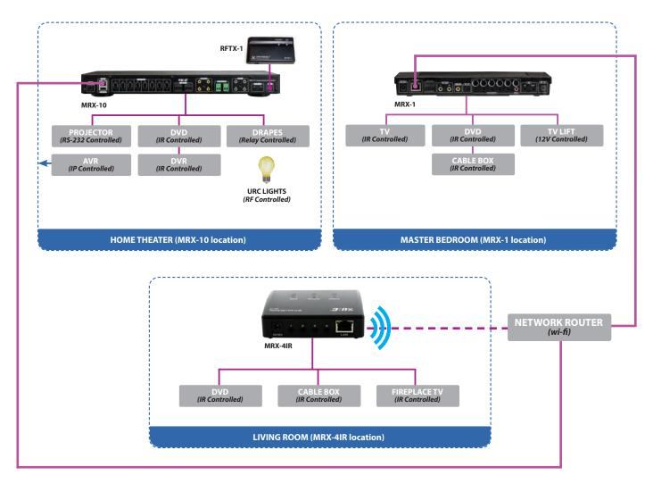
Note: The MRX-10 Advanced Network System Controller can route commands to the proper MRX unit provided each MRX unit is connected to the same Local Area Network (LAN).
