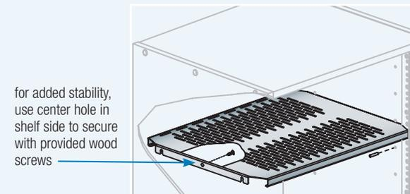
for added stability, use center hole in shelf side to secure with provided wood screws
