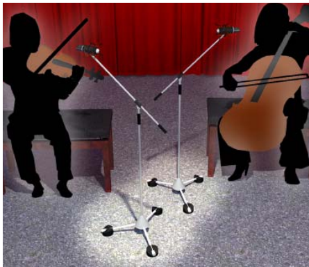
TriPads isolating celo and violin mics on a hollow and resonant stage.
