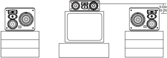
This placement provides a wide spread in sound, supplemented by the center channel speaker.
