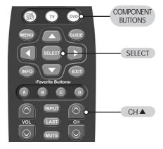
**STEP 3:** Press either the TV or CBL/SAT button that you want to use as the source of channel control. The component LED will blink two times to confirm it is saved.
