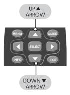
STEP 3: Point the URC-SR3 remote control toward the component and press the UP ▲ arrow (or DOWN ♥ arrow) button once. Each time the UP ▲ or DOWN ♥ arrow button is pressed, the code will count up (or down) one code number and send a Power OFF signal. When the correct code is sent out, the component will turn off. **STEP 4:** Once you have found the right code number and the component has turned off, press the POWER button on the URC-SR3 remote to turn the component back on.
