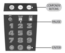
**STEP 3:** To exit Erase mode, press and hold both the component button and the ENTER (ENT) button at the same time until the component LED light blinks three times.
