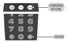
**STEP 2:** Press and hold the button you want to erase for two seconds. The component LED light will blink twice to confirm the erasure.
