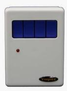
**The WPT-03 Wireless UHF Pendant Transmitter** is designed to send pre-programmed text messages directly to a designated pager or LED display.
