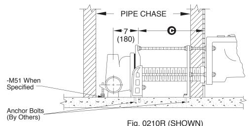
NOTES: The Installer Shall Observe and Maintain the Proper Mounting Centers of the Nipples and Studs.
