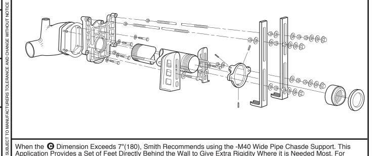
When the **G** Dimension Exceeds 7"(180), Smith Recommends using the -M40 Wide Pipe Chasde Support. This Application Provides a Set of Feet Directly Behind the Wall to Give Extra Rigidity Where it is Needed Most. For Double (Back to Back) Installations, Specify Whether the -M40 Variation is Required on One Side or Both Sides. When Ordering the **G** Dimension Must be Specified.
