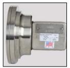
Mid-West Model 105 bellows design provides a simple, compact, accurate, direct-acting, low range differential pressure level indicator. Accuracy ±1% of Full Scale
