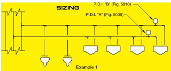
Find fixture unit weight of each fixture using Table 1. Total the fixture units weights for both hot and cold branches.
