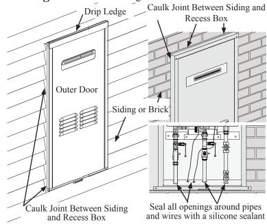
**Warning** - All openings in the bottom of the recess box must be sealed to prevent water infiltration in to the wall. Failure to do so could result in damage to the wall.
