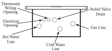
**Plumbing and Piping** - See Figure 5 for Pipe Locations. Follow all instructions in the Use and Care Manual for installation of gas and water lines. Holes are provided in the bottom of the recess box for all piping and wiring. These holes line up with the fittings on the bottom of the water heater.
