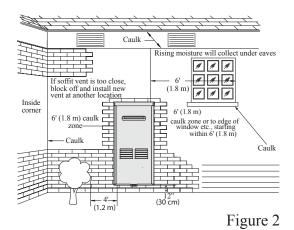
**A**WARNING: Moisture in the flue gas will condense as it leaves the vent terminal. In cold weather this condensate can freeze on the exterior wall, under the eaves and on surrounding objects. Some discoloration to the exterior of the building is to be expected. However, improper location or installation can result in severe damage to the structure or exterior finish of the building
