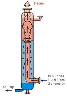
The Clayton separator is built to ASME Section 1 standards.
