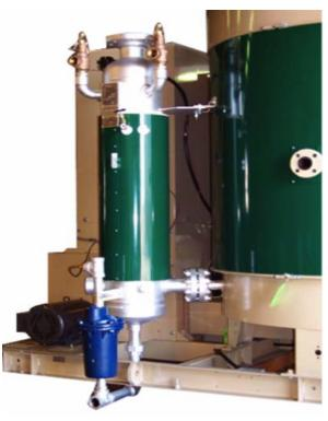
The Clayton 99.5% quality steam separator is ideally suited to projects where high quality steam is required to provide optimum performance in the steam system. Typical applications include Food Processing and Conditioning (such as Grain & Feed Mills) where water content of the product requires high quality steam and temperature sensitive heating of integral manufacturing components such as the rolls in a corrugator.
