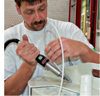
Wire welding using the compact, light WELDING PEN R.
