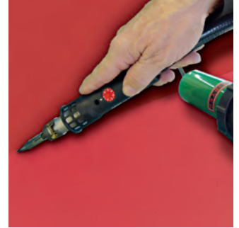
LABOR S, used in connection with MINOR as an external air supply.
