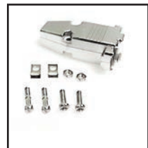
30-553M (Nickel) 30-553M-G (Gold) DB9, DB15HD metal housing for 10-11mm cable, with hardware. 2-piece construction, for use with DB9, DB15 type connectors.
