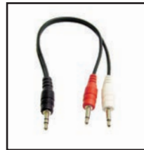
35-560 3.5 mm stereo plug to two 3.5 mm mono plugs, shielded. 10" long.
