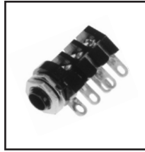
30-397 1/4" Audio Jack. Open Circuit 3-Conductor. 3/8" bushing, Mounts in .355" hole.
