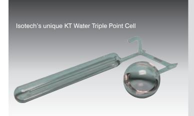
Reverting to the very first designs of water triple point cells, Isotech produce a cell with Isotopic analysis, a McLeod gauge to assess any trapped air and an attached flask where the cell's water can be transferred and redistilled. By accounting for these sources of uncertainty we claim that this cell represents the ultimate reference for those requiring cells as close to ITS-90 as possible. Please ask for a copy of a comprehensive report describing the cell, its operation and performance.
